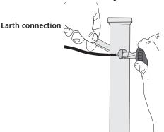
NOTE: Connect additional earth stakes with lead-out cable if required
