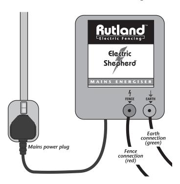
**STEP 1: Mount Energiser** *IMPORTANT: Mount in an inside location or in a waterproof enclosure*
